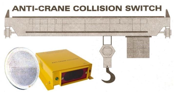
AntiCrane Collision Switch for two over head cranes on the same rail. These units are installed on two cranes on the same rail approaching each other. With these units, the two cranes on the same rail will never collide with each other & thus the damage caused due to collision can be saved. The minimum distance in between two cranes will always be maintained, and the cranes will be able to move away from each other but not closer.
